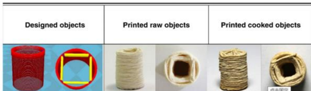
Figure 13: Shape of 3 D printed cereal-based samples before and after baking. Adapted from (Severini et al., 2016).
